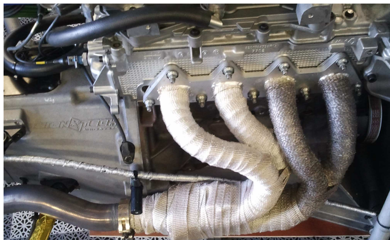
Example of exhaust thermal protections now forbidden
