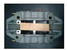
• Place an air blow gun in the hole of the caliper pipe and pressurize to push the pistons out.
