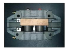
• Remove the block of wood and remove the springs
